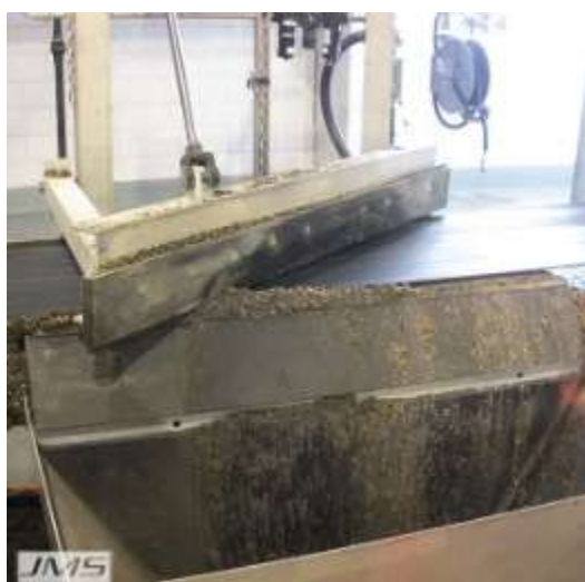
Figure 4-14. Belt Conveyor Plow Courtesy of Jim Myers and Sons
