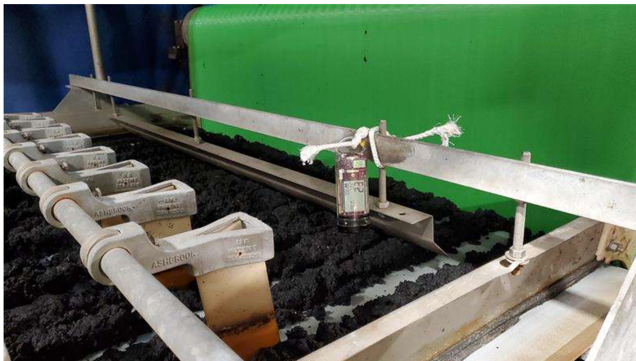
Figure 5-1. Belt Filter Press Acrulog H 2 S Monitoring Lemay WWTF Odor Sampling
