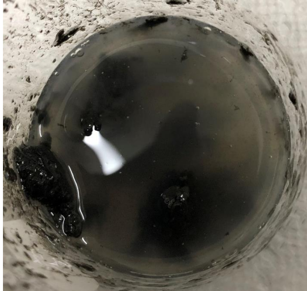
FIGURE 8 – OVERDOSE EXAMPLE FOR THE C-6267 POLYMER AGAINST THE BISSELL SLUDGE
