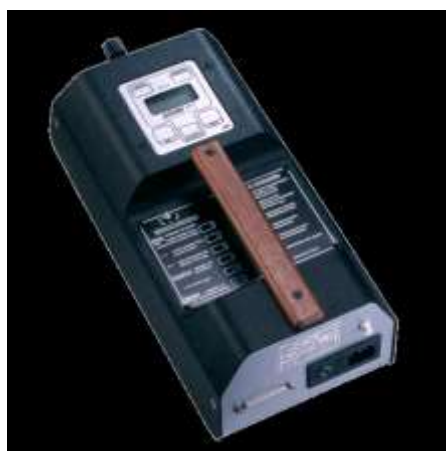
Figure 2-1. Jerome 631-X analyzer used for field H_2S measurements
