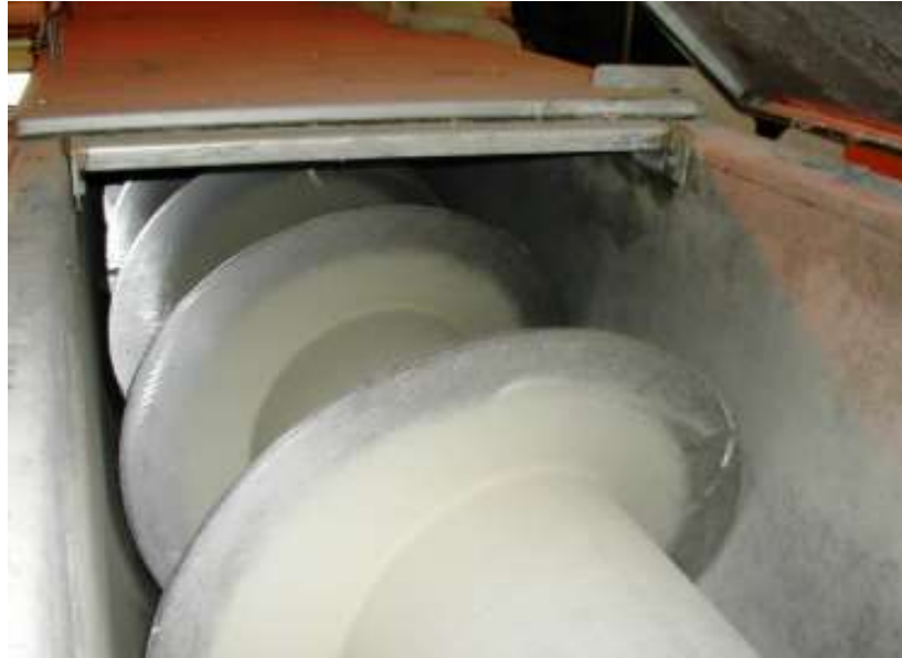
Figure 4-12. Screw Conveyor Courtesy of Custom Conveyor
