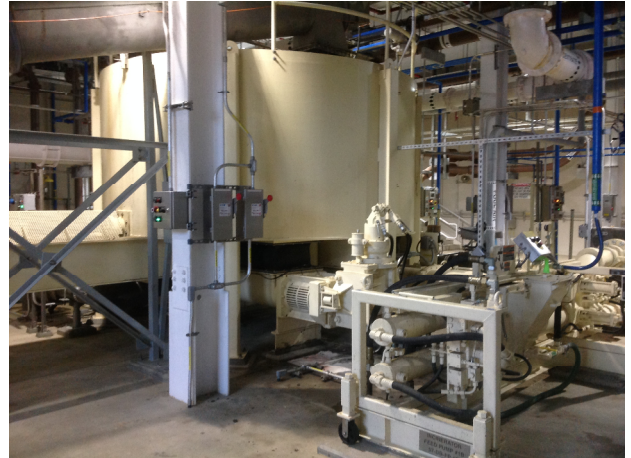
Figure 9. Example of Sliding Frame Bin Downstream of Dewatering Centrifuges at NEORSD's Southerly
