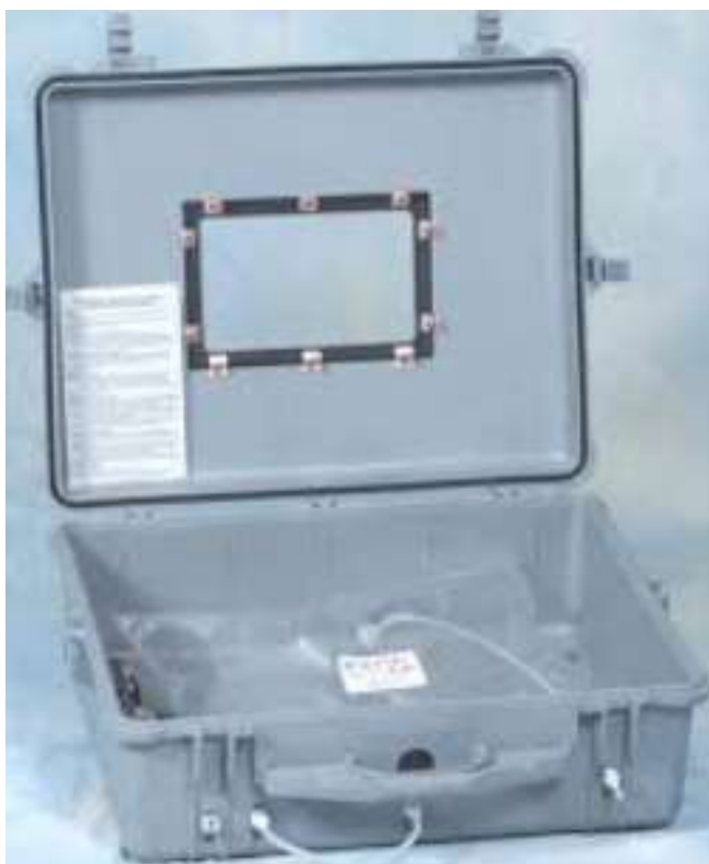
Figure 2-3. Vacuum chamber for Air Sampling using Tedlar bags
