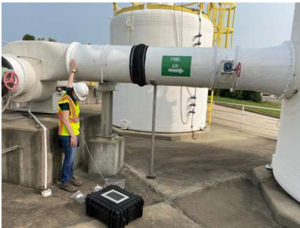
Figure 2-3. Vacuum chamber apparatus for air sampling
