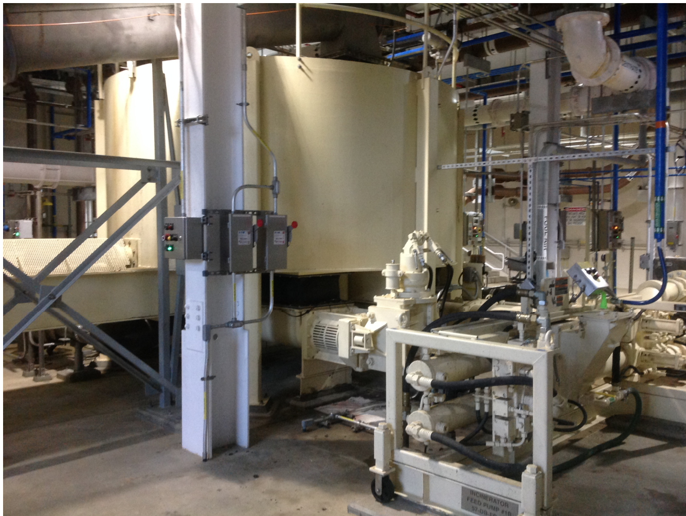
Figure 4. Example of Packaged Cake Collection Bin and Hydraulic Piston Pump
