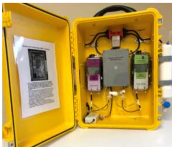
Figure 2-2. Installed Acrulogs Inside an LRSS
