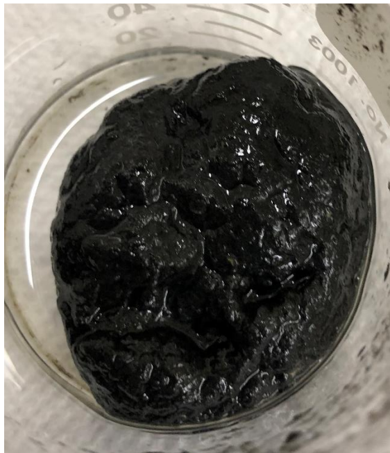
FIGURE 7 – A PELLET OF SLUDGE AFTER FLOCCULATION WITH 16 LBS/TON ACTIVE OF K274 FLX AGAINST SLUDGE FROM BISSELL POINT WWTP
