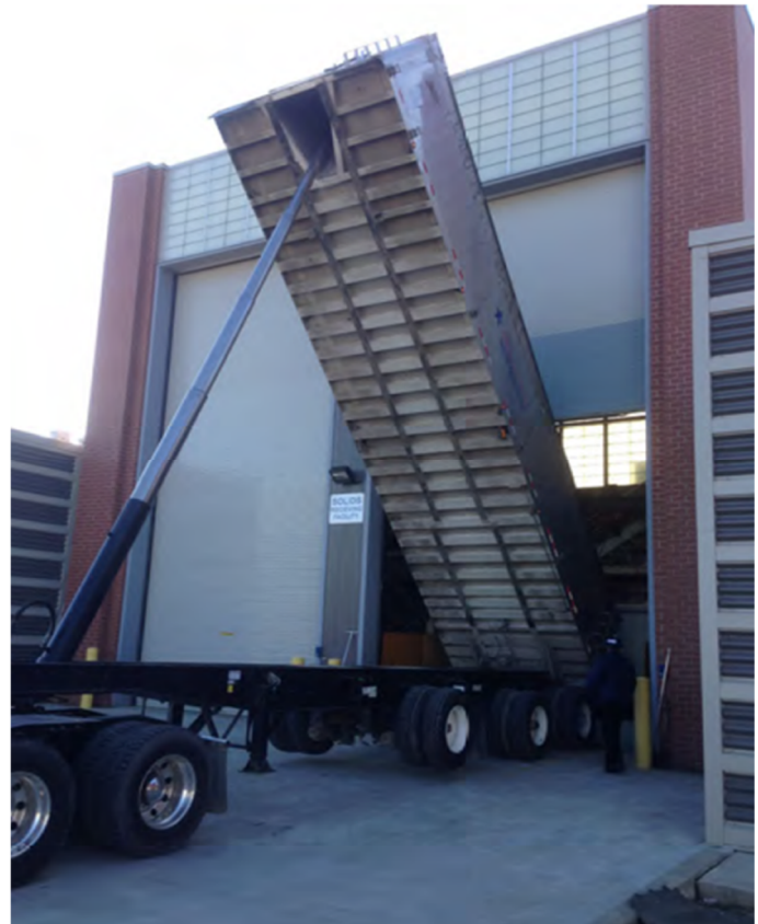
Figure 6. Example of Truck Unloading for Indoor Cake Receiving Station at GEB WWTP
