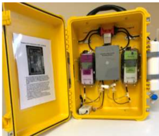
Figure 2-2. Installed Acrulogs inside an LRSS
