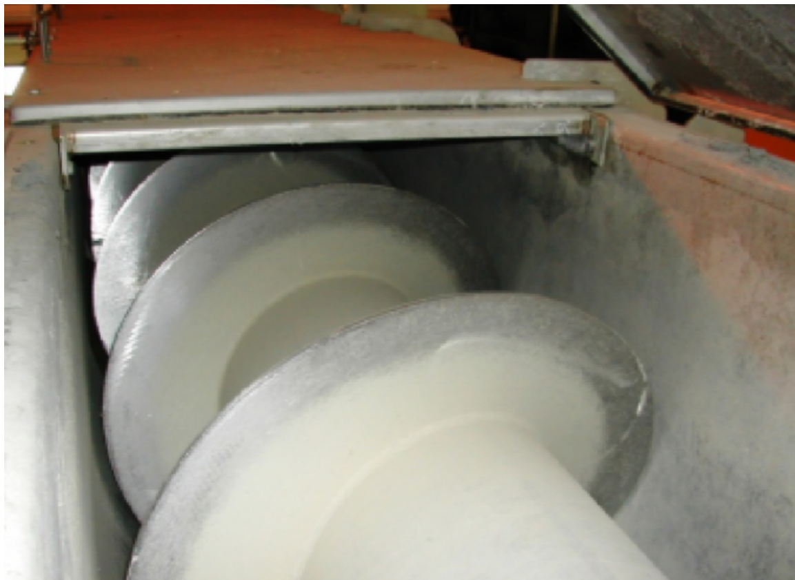
Figure 2. Example of Typical Shafted Screw Conveyor
