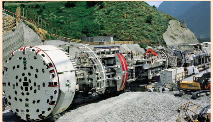
Large-diameter TBM with the "business end" or cutter head at left, and the support or "trailing" gear behind it.
